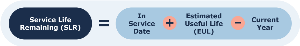
Figure 7 Service Life Remaining Calculation
