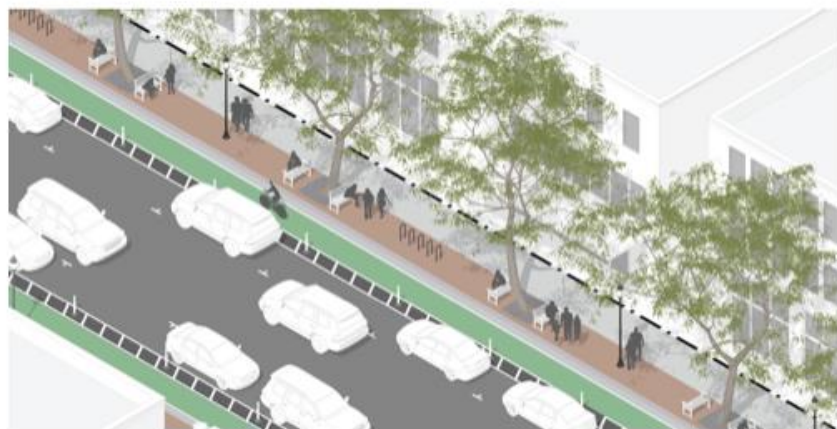
Figure 31 – Planting and Furnishing Area Conditions
