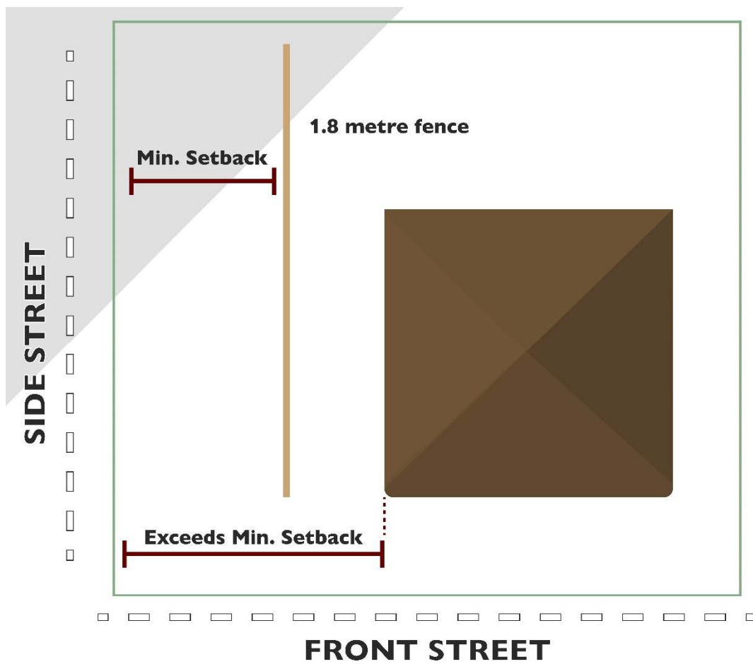
Figure 3 - Exterior Side Yard that Exceeds Minimum Setback, 1.8 metre high fence
