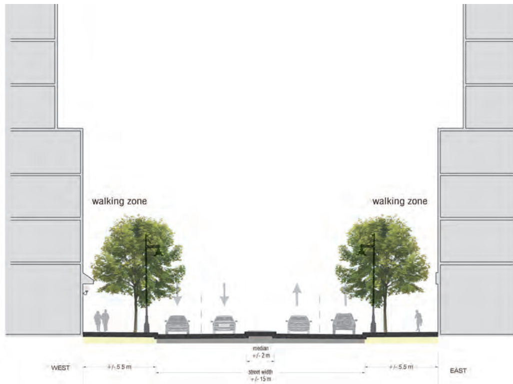
FIG 19 : PROPOSED GRANDIN RD SECTION
