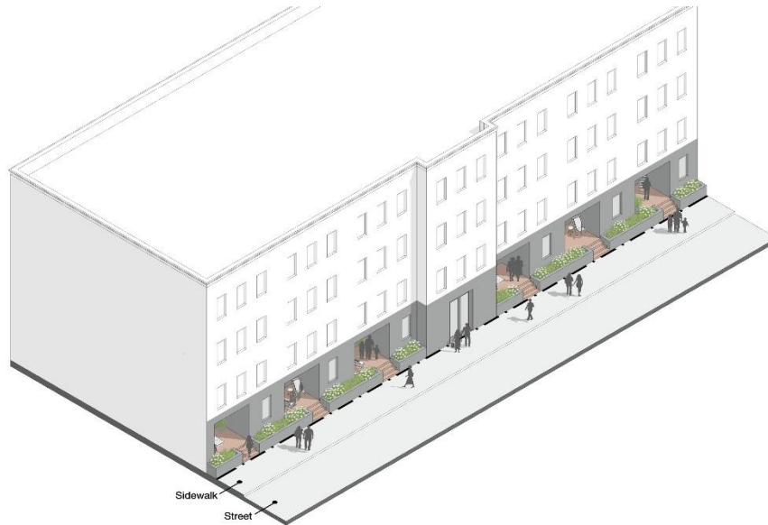
Figure 4 – Embedded Porch Frontage Design Elements
