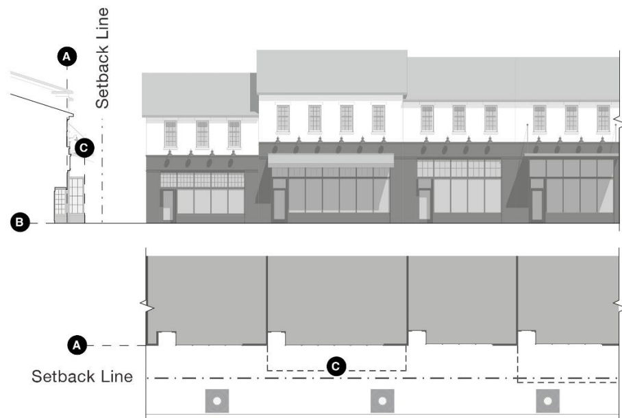
Figure 19 – Illustrated Entry and Glazing Requirements
