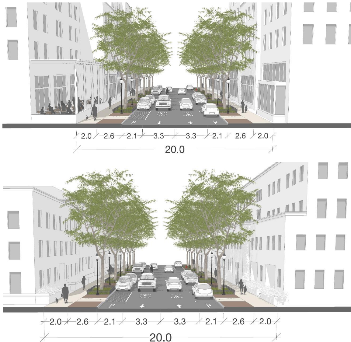
Figure 29 – Typical Framework Street Section
