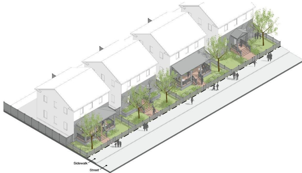
Figure 6 – Fenced Yard Frontage Design Elements
