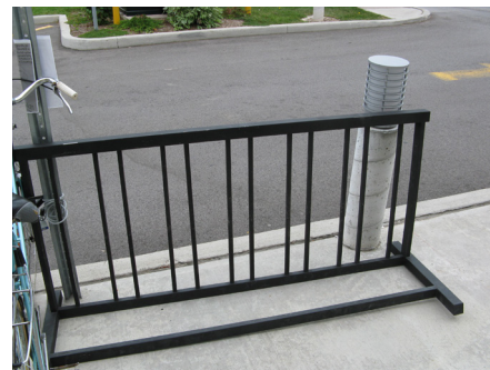
Wheel-only supportive bicycle racks are not permitted.
