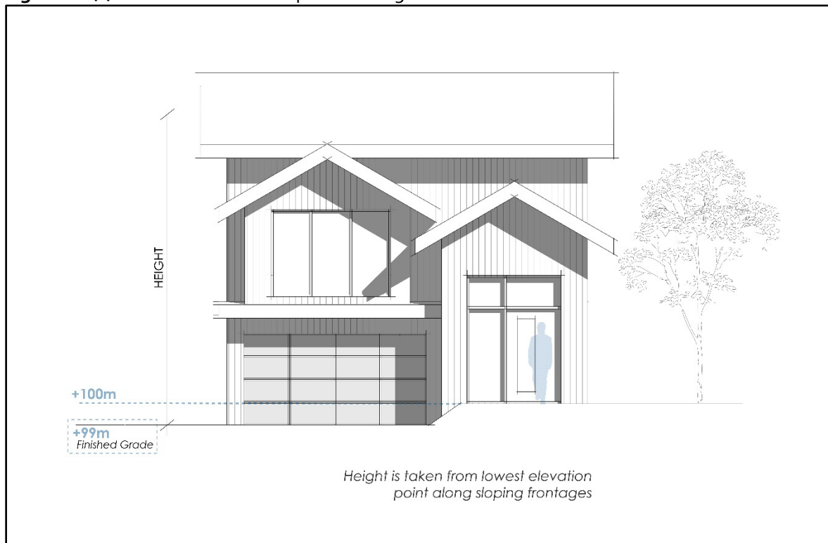
Figure 5.3(c) – Finished Grade: Sloped Fronting Road
