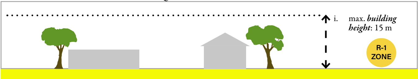
FIGURE 7. MAIN BUILDING HEIGHT REQUIREMENTS
