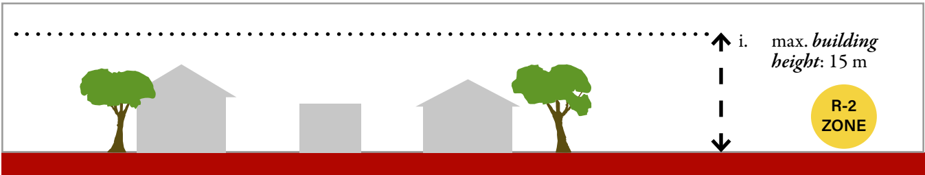
FIGURE 9. MAIN BUILDING HEIGHT REQUIREMENTS
