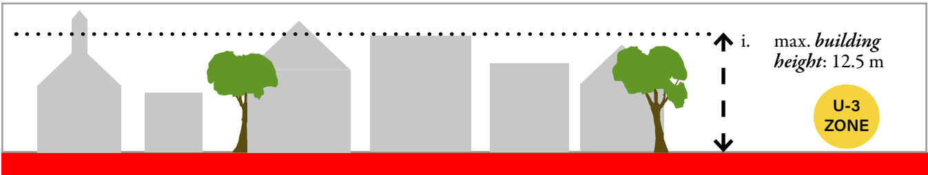
FIGURE 18. MAIN BUILDING HEIGHT REQUIREMENTS
