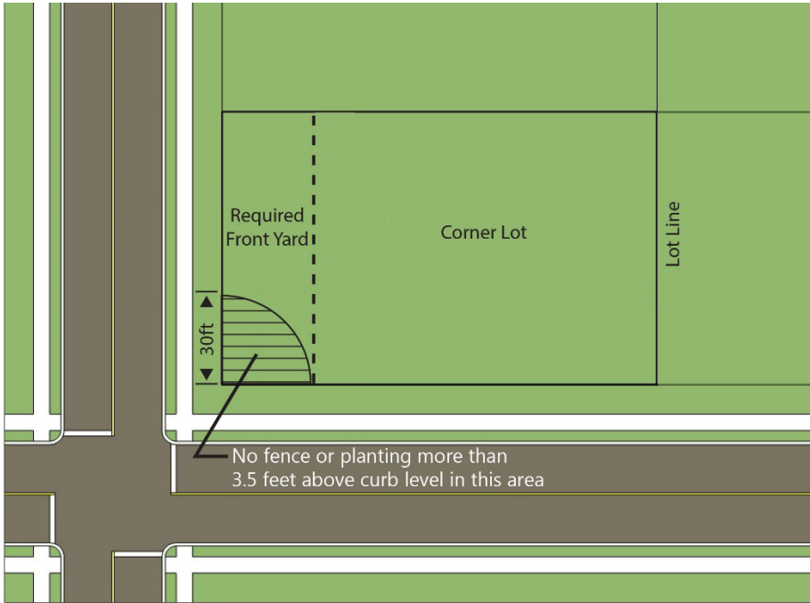
Figure 5: Visibility clearance at intersections
